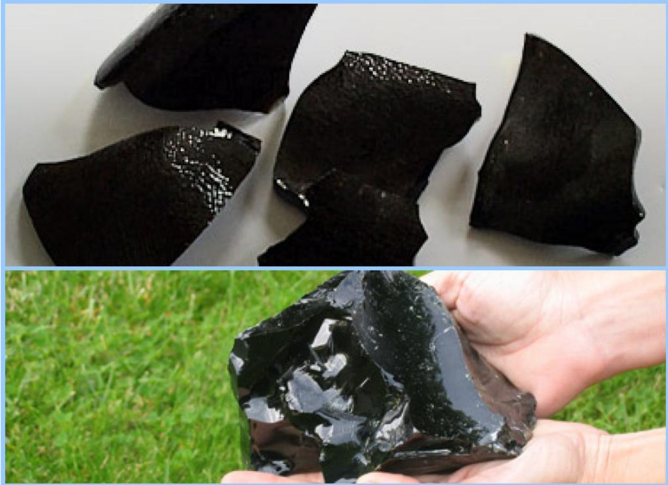
Diagram 32: Vitrified, glass-like, inert slag
